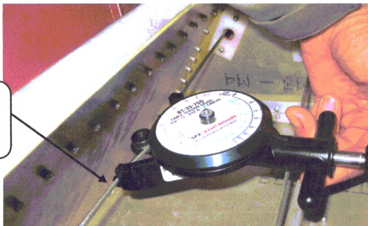
Photo of tensiometer on left Aileron cable seen from pilot seat (see flap motor on right). Repeat process on right aileron cable, behind passenger seat.
